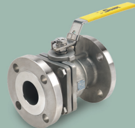
150#, 300#, 600# Flanged Ball Valves Full & Reduced Port Carbon Steel, 316 Stainless & Alloy 20 1/2" - 12"
