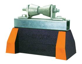
The HBS-R Series are designed for superior support of gas and refrigeration pipes. The roller allows for longitudinal movements of the pipe. This support is suitable for most types of roofing material or other flat surfaces.
